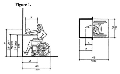
NOTE: x shall be  $\leq 25$  in(635 mm); z shall be  $\geq x$ . When x < 20 in(510 mm), then y shall be 48 in(1220 mm) maximum. When x is 20 to 25 in(510 to 635 mm), then y shall be 44 in(1120 mm) maximum.
