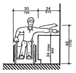
35.1.17 The highest operable part of controls, dispensers, receptacles, and other operable equipment shall be placed within at least one of the reach ranges outlined in paragraphs (15) and (16) of this subsection.
