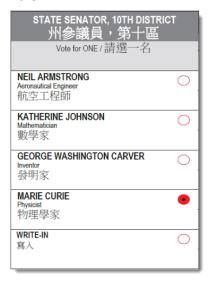
Figure 4-2: Contest marked with 7% Marginal Fill Factor
