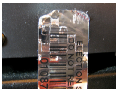
Figure A-2: Evidence of Tampering: Peeled and Reapplied
