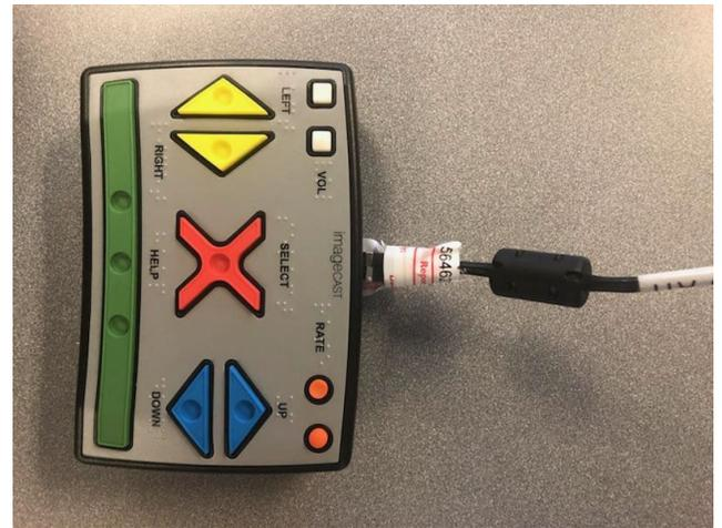
3. ATI USB Cable (ICX Samsung Only) – Seal the USB connection of the ATI Cable to the bottom of the ICX so that the seal covers both ends of the cable.
