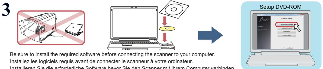
Be sure to install the required software before connecting the scanner to your computer.
