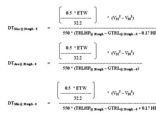
(D) The maximum and minimum time limits for the off-dynamometer coast-down window at 20 mph (DTMax @20mph-20 , DTMin @20 mph-20 ) for dynamometers with 20.0-inch rolls shall be calculated by the following equations. The TRLHP and GTRL used in these calculations shall be determined from the same vehicle/engine category used to determine the 50 mph off-dynamometer target coast-down time.
