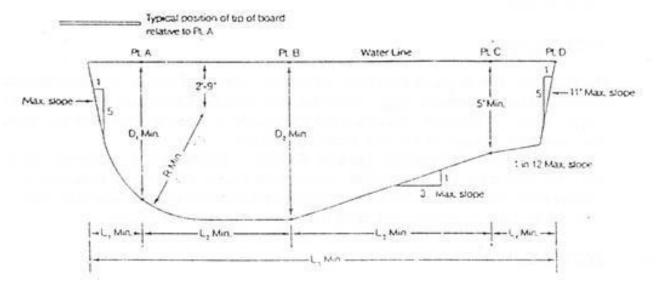
Note: L4 Is a minimum dimension to allow sufficient length opposite the board. This may of course be lengthened to form the shallow portion of the pool.
